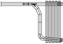
■ Straight run with 135-degree parallel stack.
